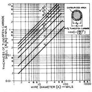
Fig. 4-Carbide shell thickness versus wire diameter and per cent carbide.
