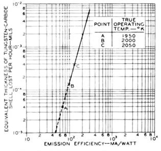
Fig. 3-Carbide loss versus operating temperature.
